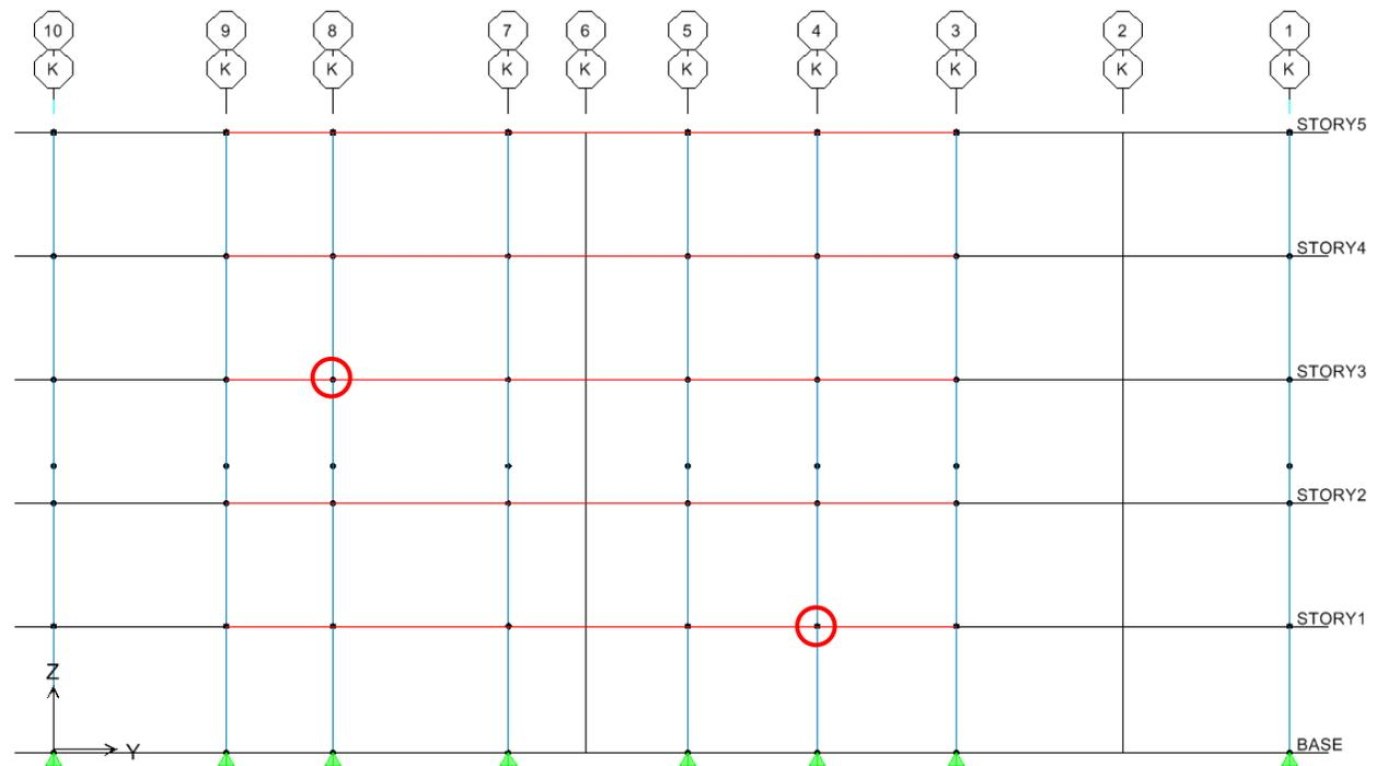
Figure 34: N-S Frame - Selected Joints for Moment Connection Design/Detailing
