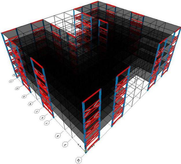
Figure 25: 3D View of Existing Braced Frames ETABS Model
