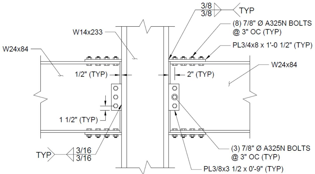
Figure 35: Bolted Flange-plated FR Moment Connection to Second Floor Beams at J-10
