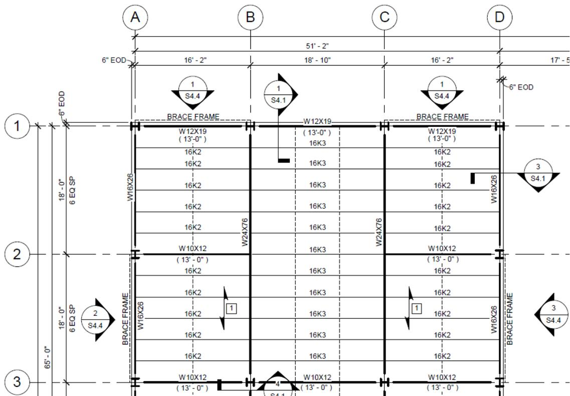
Figure 4: Typical Floor Framing Plan (Enlarged)
