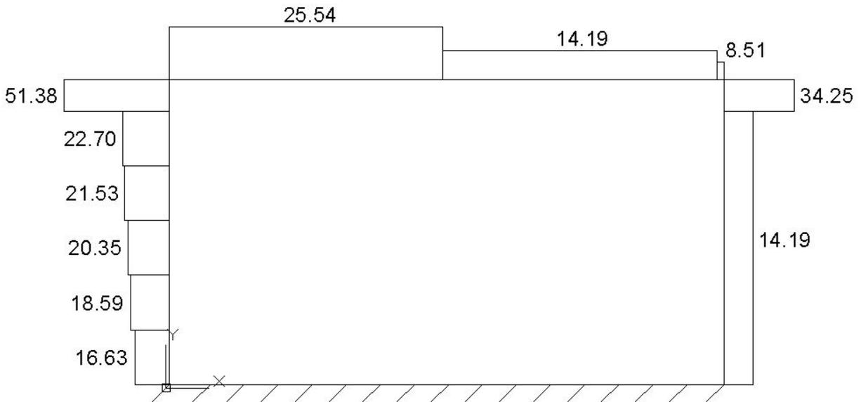
Figure 13: N-S Wind Pressure Diagram
