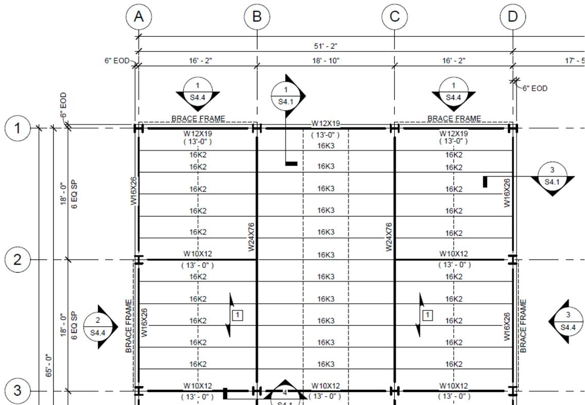
Figure 4: Typical Floor Framing Plan (Enlarged)
