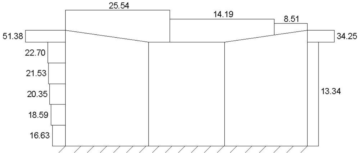
Figure 17: E-W Wind Pressure Diagram
