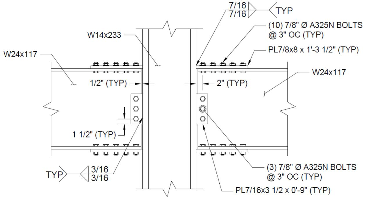
Figure 36: Bolted Flange-plated FR Moment Connection to Second Floor Beams at K-4
