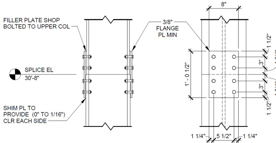
Figure 31: Typical Column Splice Detail
