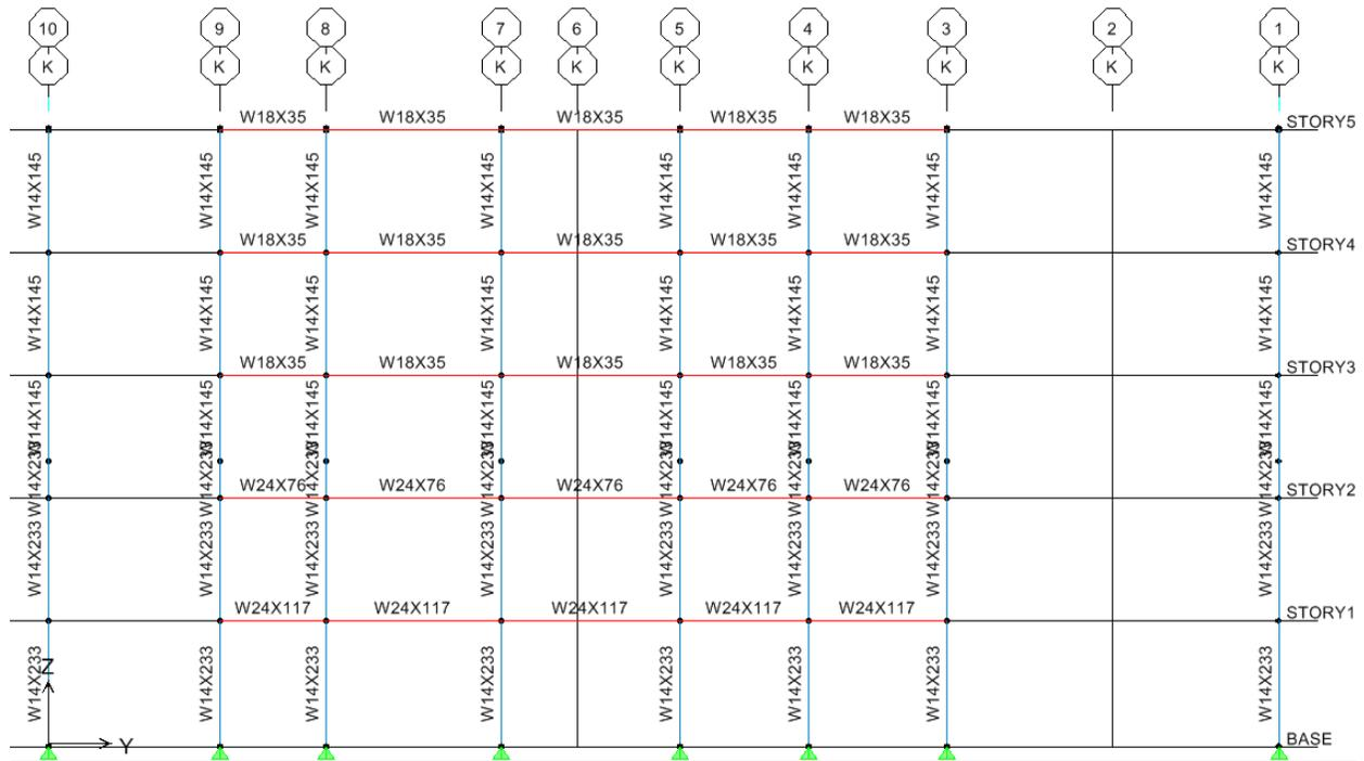
Figure 30: N-S Rigid Frame Member Sizes
