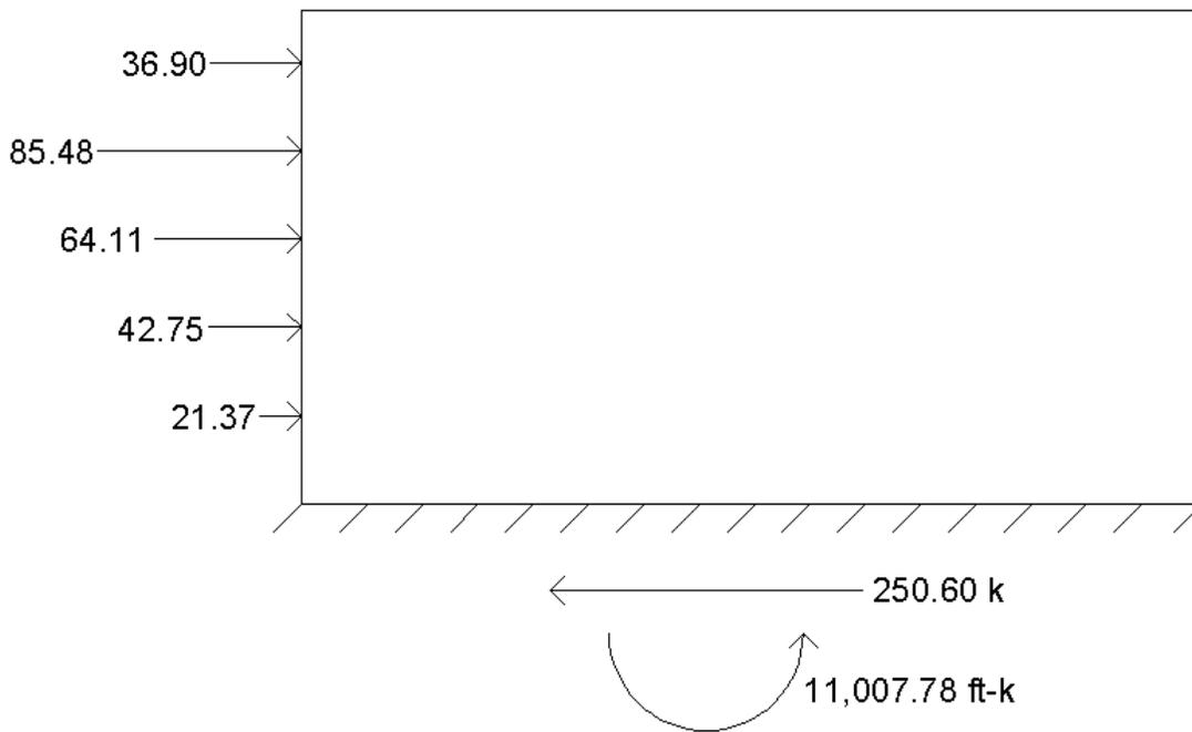
Figure 20: Seismic Force Diagram
