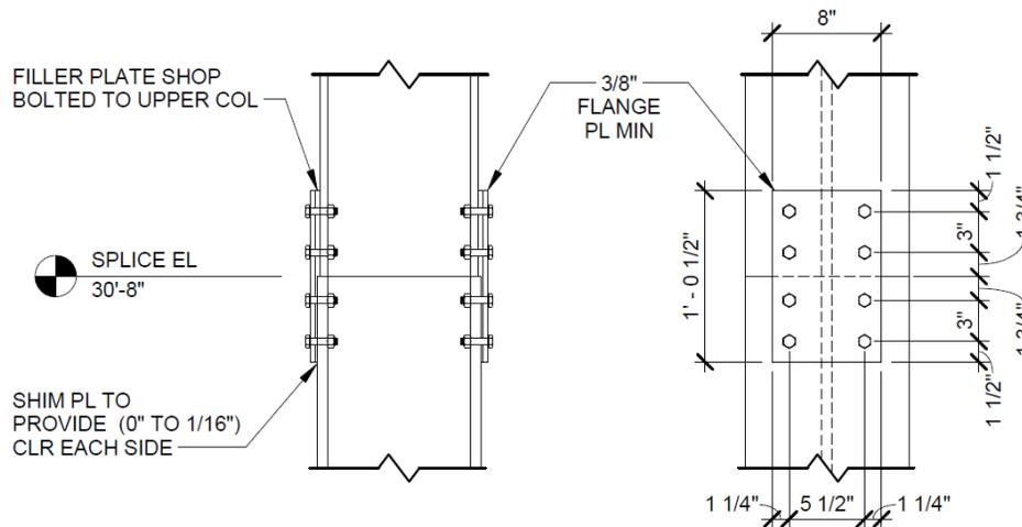
Figure 31: Typical Column Splice Detail
