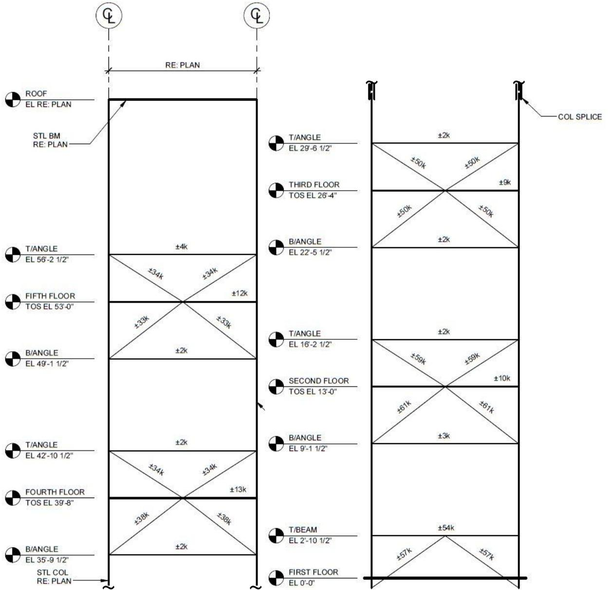
Figure 7: Typical Braced Frame Elevation
