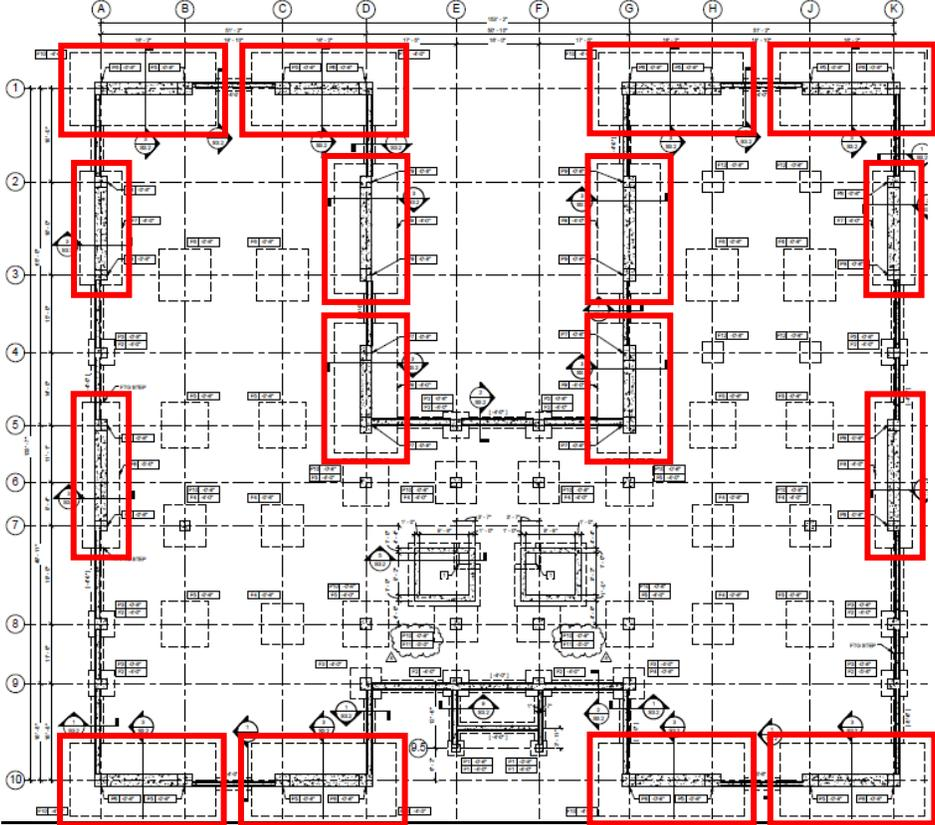
Figure 3: Braced Frame/Combined Footing Locations
