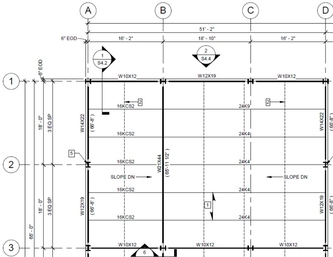
Figure 5: Typical Roof Framing Plan (Enlarged)
