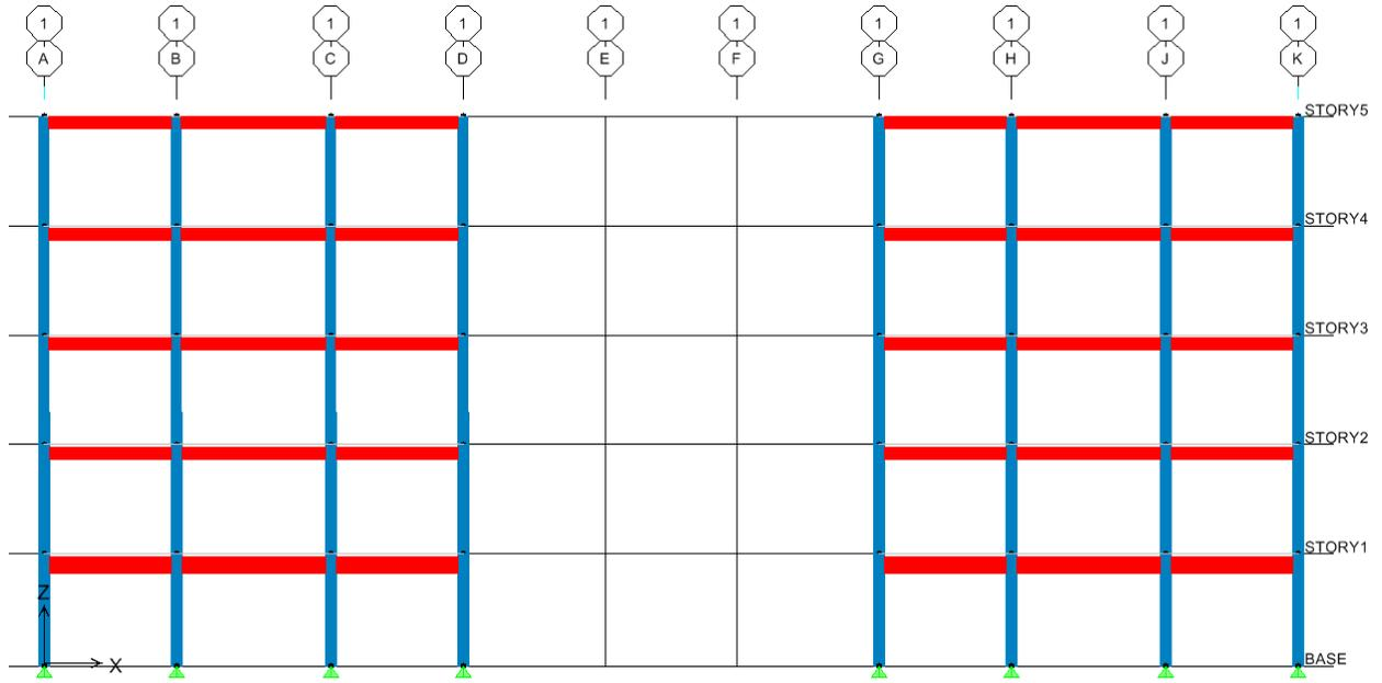
Figure 27: E-W Rigid Frames at Grids 1 and 10
