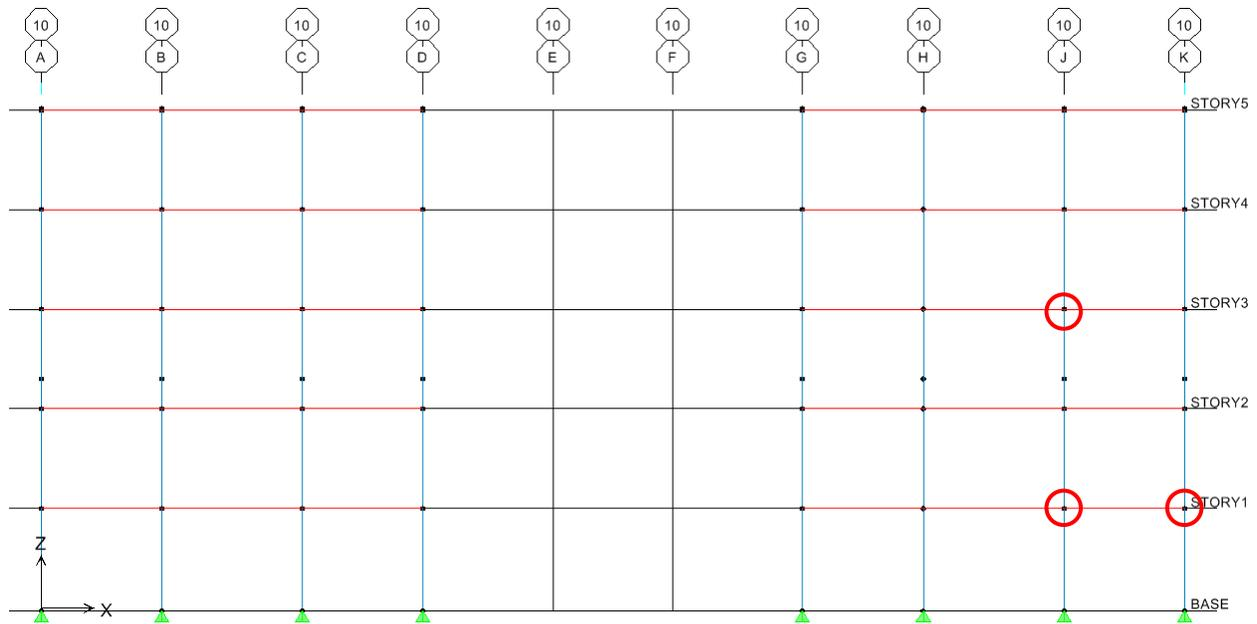
Figure 33: E-W Frame - Selected Joints for Moment Connection Design/Detailing
