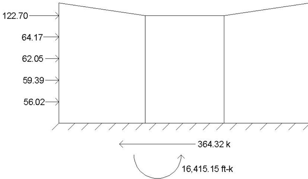
Figure 18: E-W Wind Force Diagram
