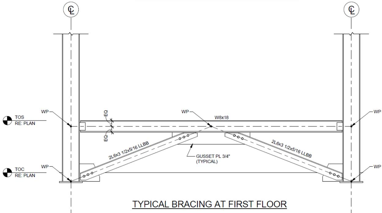
TYPICAL BRACING AT FIRST FLOOR
