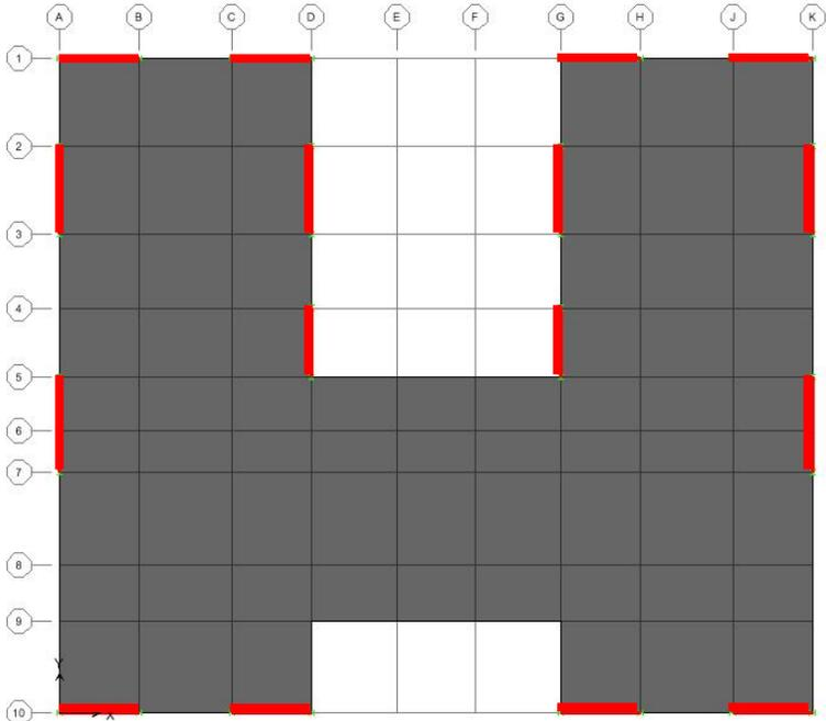
Figure 23: Existing Braced Frame Layout
