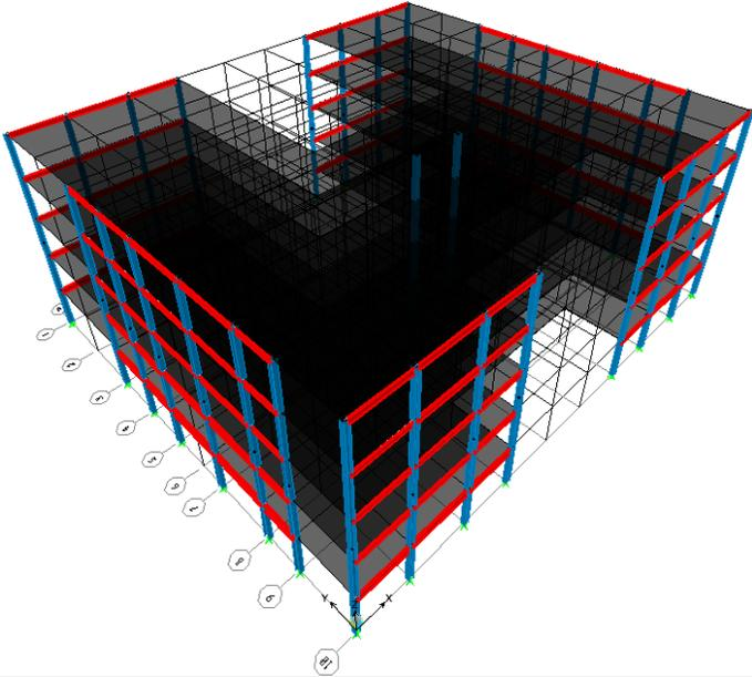
Figure 26: 3D View of Proposed Moment Frames ETABS Model
