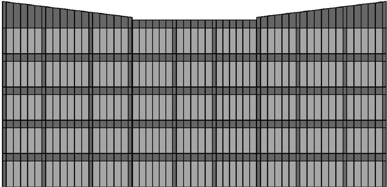
Figure 40: Front Façade Elevation showing Proposed Curtain Wall System
