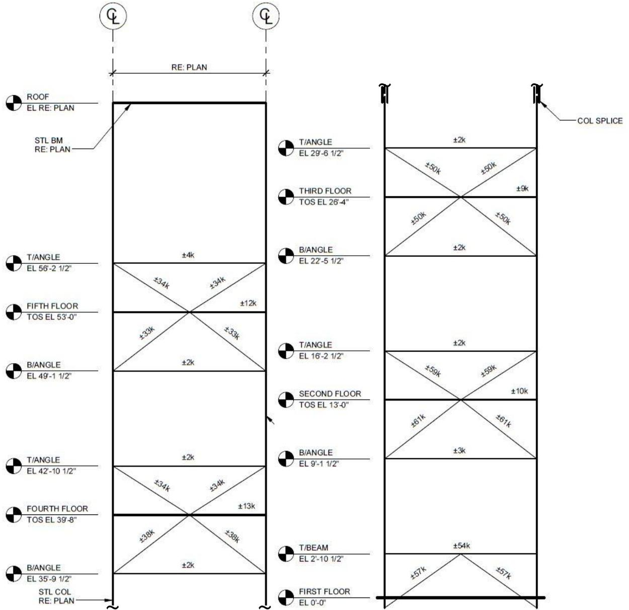
Figure 7: Typical Braced Frame Elevation
