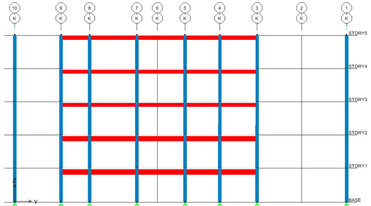
Figure 28: N-S Rigid Frames at Grids A and K
