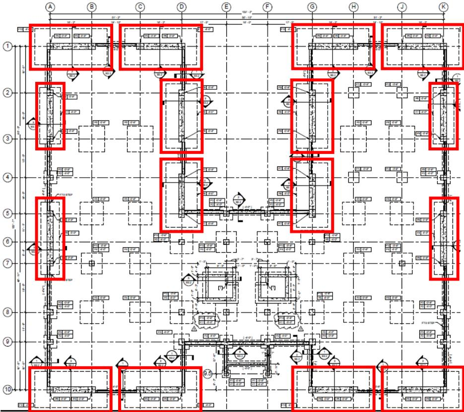
Figure 3: Braced Frame/Combined Footing Locations
