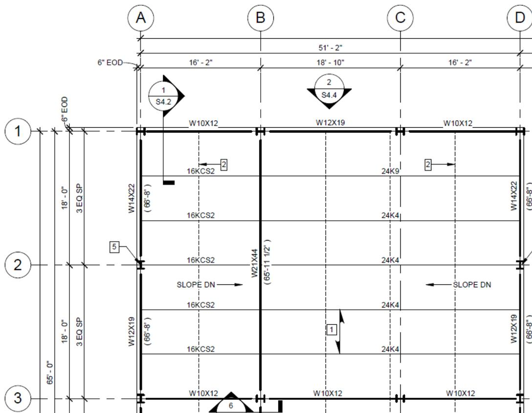
Figure 5: Typical Roof Framing Plan (Enlarged)
